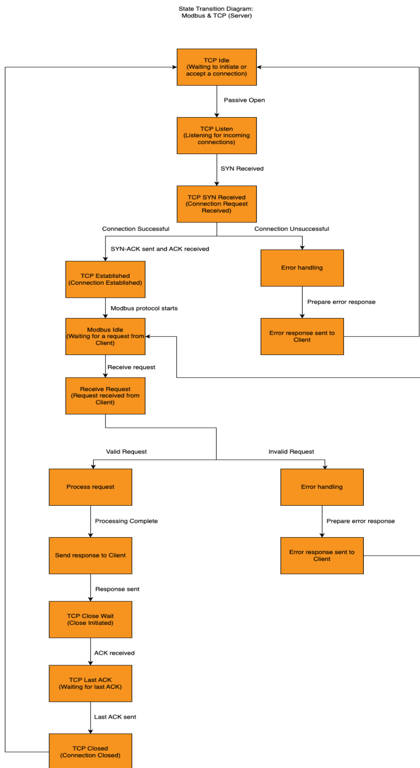
Figure 26: Transition diagram for Modbus TCP Server
