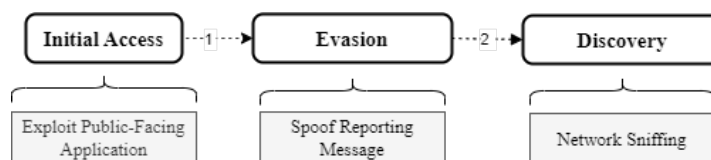
Figure 15: Steps - Pathway of AV VPN Server DNS Spoofing
